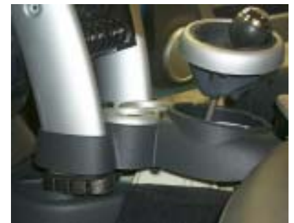
Shifter bezel lifted off, and shifting of pillars to expose mounting screws.
